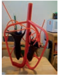
Fig. 9 Wax sprues used during the sculpture fabrication process
